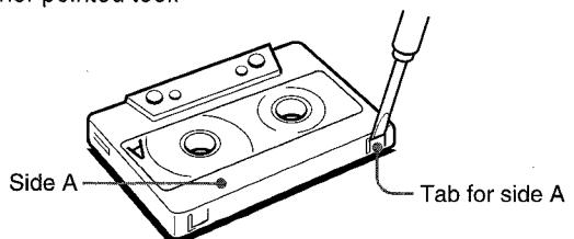
To record on the tape again, cover the tab openings with adhesive tape, etc.
